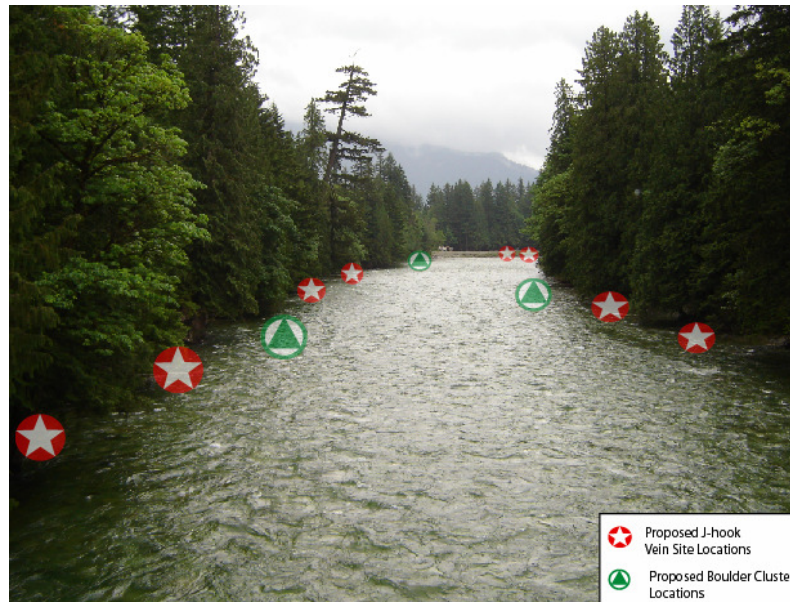
Figure 2. Proposed locations for the j-hook vein structures and boulder clusters downstream of the Morris Valley Bridge.
