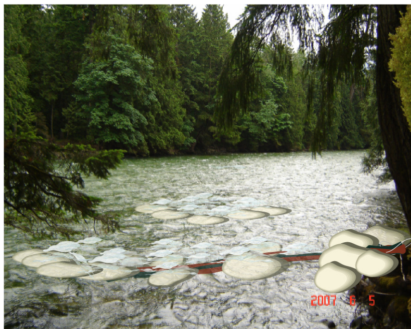
Figure 5. Conceptual site drawing of proposed j-hook and boulder cluster site on the lower Chehalis River.
